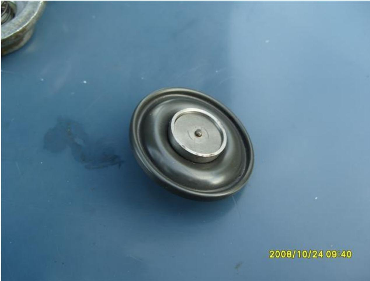
Put the new diaphragm in the top cover - make sure it's the right way round as shown.
