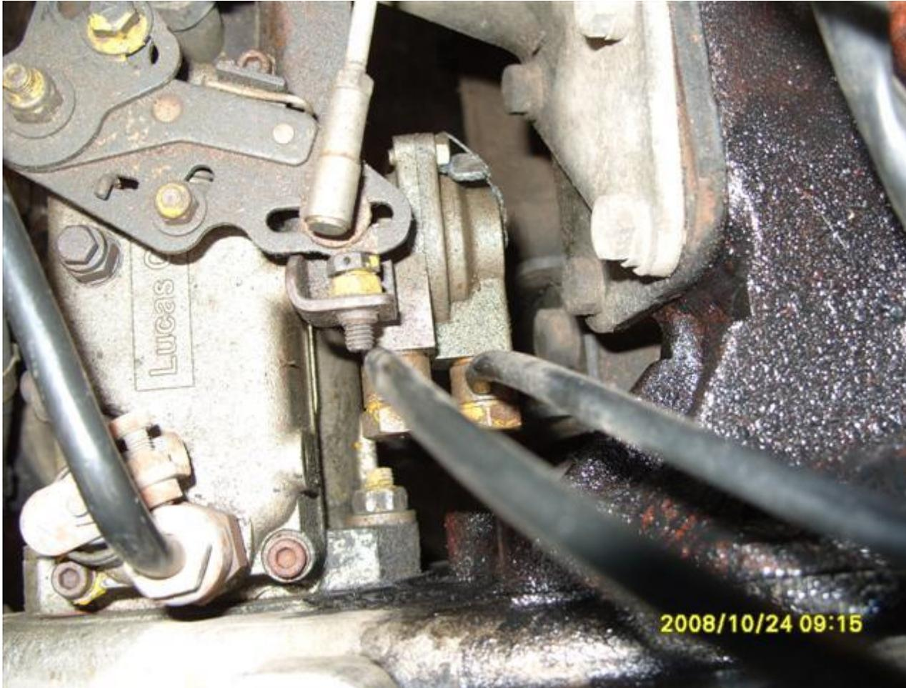
There are two pipes connected to the boost housing - one goes to the spill rail, and the other goes to the turbo. Both banjo bolts are identical (5/8"). Make a note of which pipe goes where, then remove both fittings - retrieving the 2 x copper sealing washers from each.
