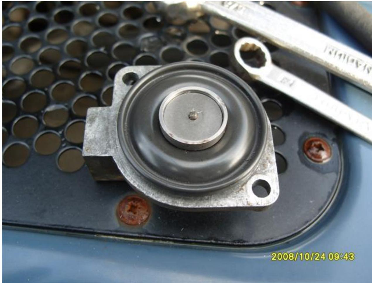
Make sure the cover is located correctly and hold it in place while you fit the two bolts - top one first. Reconnect the two pipes - making sure there's a copper sealing washer either side of the banjo fitting and don't excessively tighten the bolts - they are fine thread and will strip very easily. Start the engine - it may smoke initially, due to the fuel residue in the pipework, but this will clear fairly quickly.
