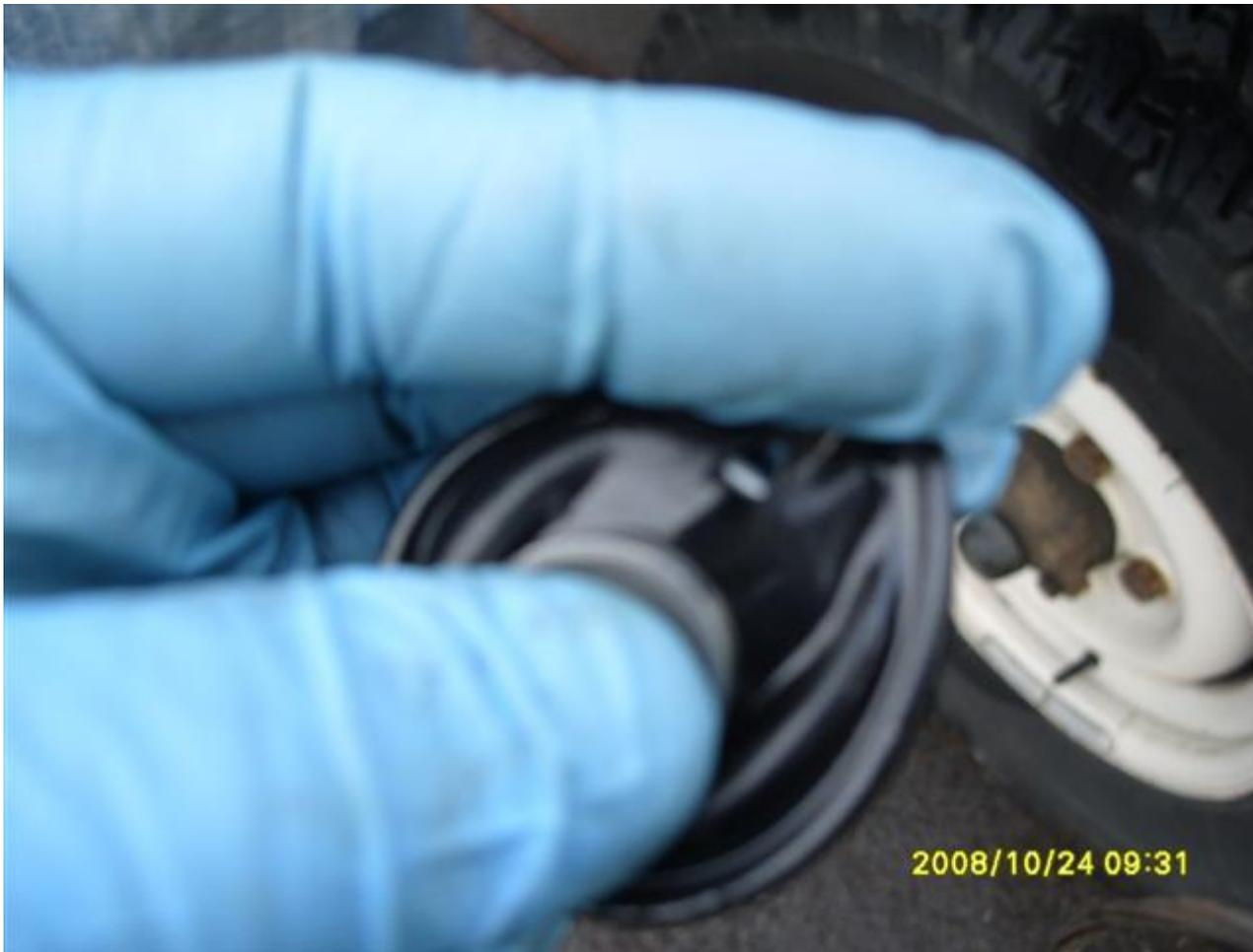
The centre pin of the new diaphragm must be the same as the old one. There's a 10mm lock nut on the back, slacken it and then turn the pin until it protrudes the same amount, then tighten the lock nut.
