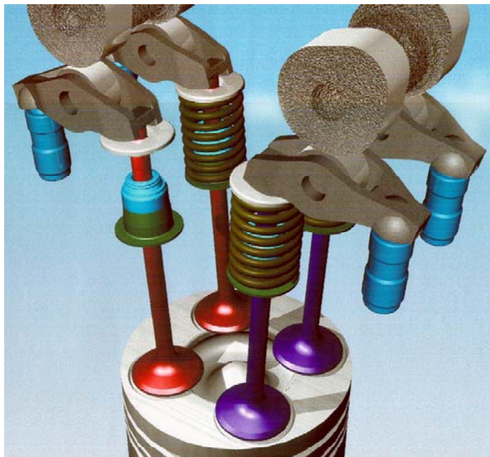
Fig. 43. Inlet and exhaust valves
