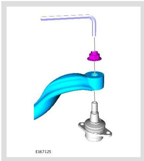
Install the ball joint to the rear lower arm.
