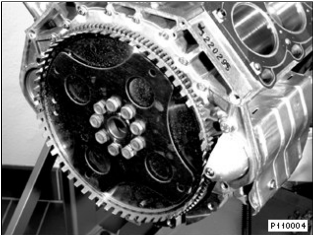
Flywheel with increment gearing
