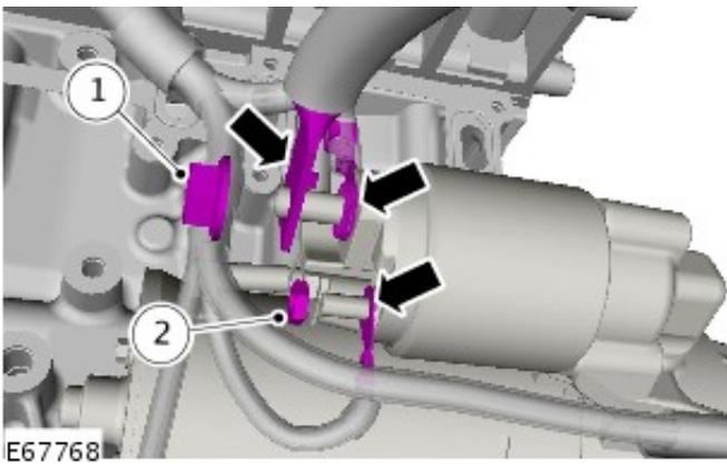
Secure the 2 battery positive cables and the ground lead to the starter motor solenoid.
