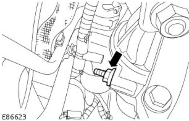
7. Remove the starter motor.
