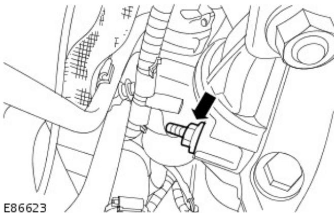
3. Secure the 2 battery positive cables and the switch lead to
