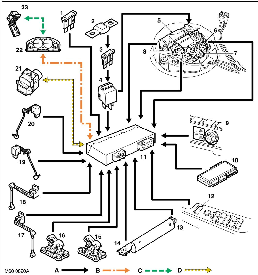
A = Hardwired connections; B = K bus; C = Diagnostic DS2 bus; D = CAN bus
