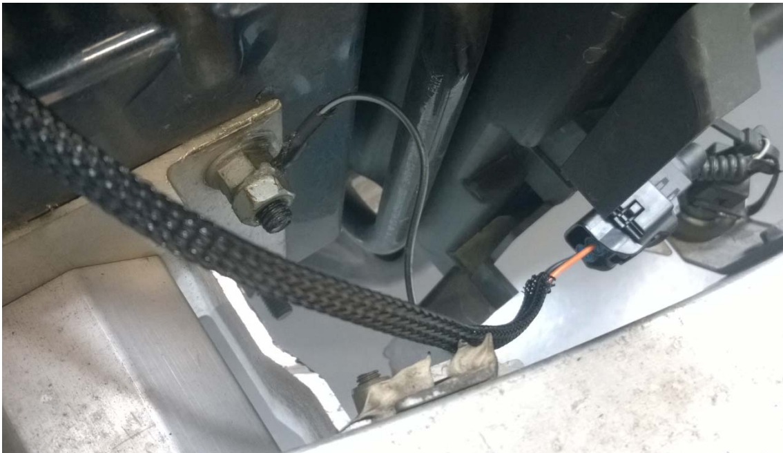
Note the earth wire fitted with 8mm nut and a little bit of silicon to stop corrosion setting in
