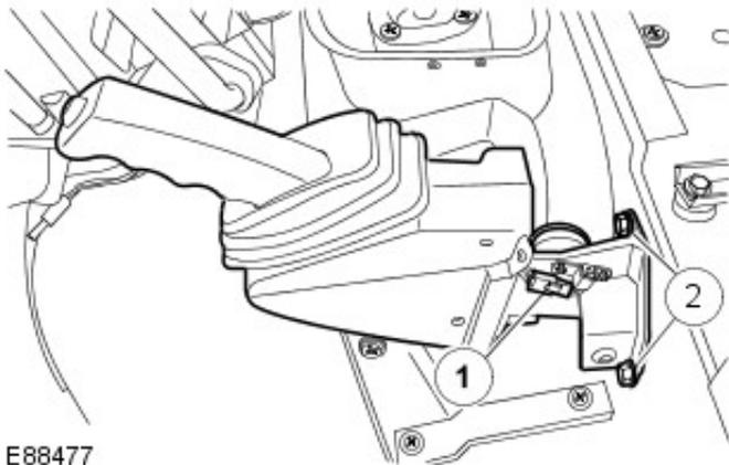
5. Remove the transmission cover panel floor covering.
