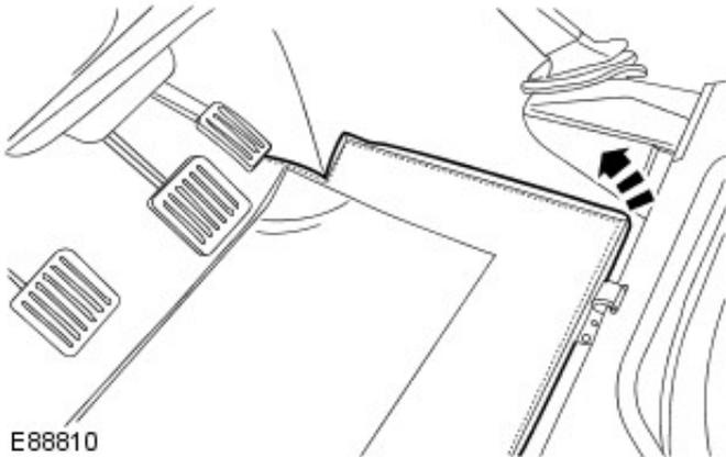
3. Release the parking brake lever gaiter.
