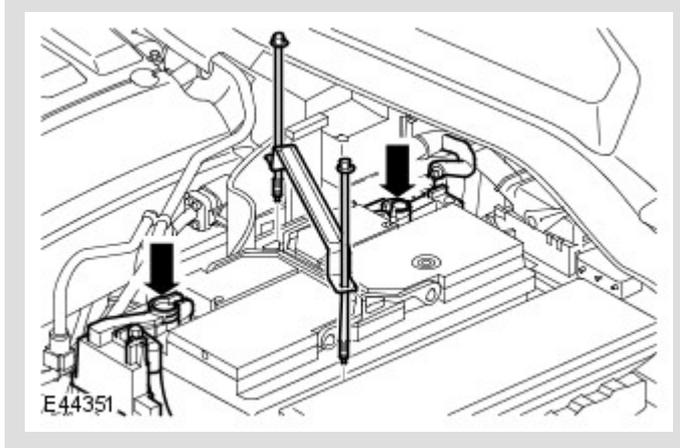
Remove 2 bolts securing the battery clamp and remove the clamp.
