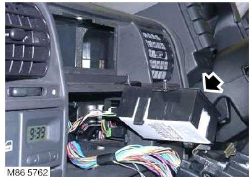
6. Remove 2 studs securing alarm receiver.
