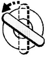
**5. Enter the FOURTH number of the code.** If the fourth number is 1, turn the key to the LOCK position once. Ensure the key is FULLY returned to the centre position.
