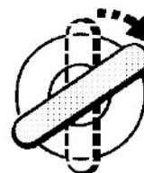
**2. Enter the FIRST number of the code.** If the first number is 4, turn the key (towards the front of the car) to the UNLOCK position 4 times. Ensure the key is FULLY returned to the centre position after each turn.
