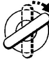
**1.** Ensure that all doors are closed, then using the key turn the driver's door lock to the UNLOCK position (towards the front of the car) and hold in this position for at least 5 seconds until the alarm sounder sounds once). Then return the key to the centre position. It is now possible to use the key to enter the separate numerical values of the four numbers that make up the emergency key access code.
