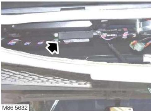
3. Remove 2 nuts securing receiver to roof panel, disconnect multiplug and remove receiver.
