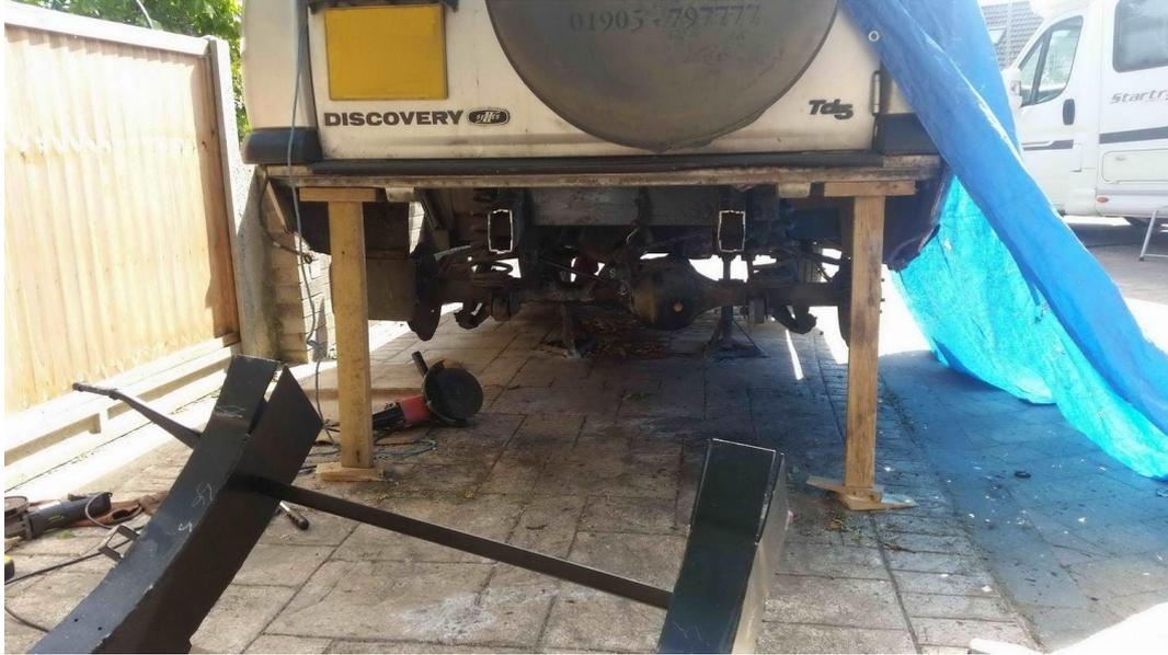
the new bit fitted well, did a trail fit, removed it cleaned up the original sections were it will weld on the refitted it and bolted it up in place
